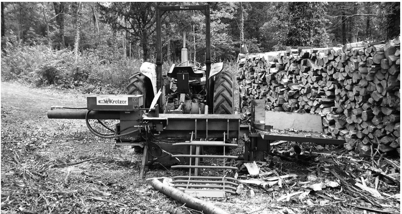
A 20 tonne force horizontal log splitter.
